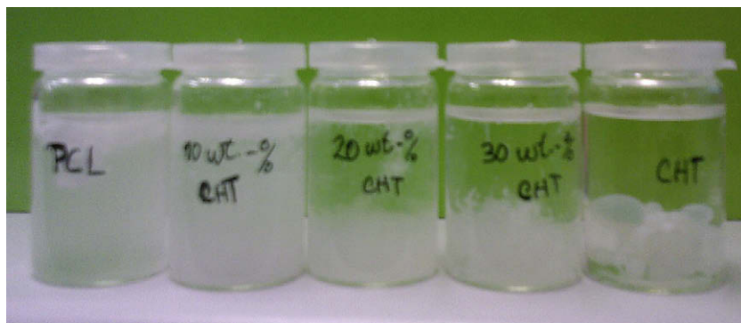
Fig. 2. Photographs of neat chitosan (CHT), polycaprolactone (PCL) and PCL/CHT blends poured in a solution containing excess of sodium tripolyphosphate.
